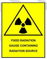
d) the area in the vicinity of a **portable** radiation gauge is designated as either a Supervised Area or a Controlled Area, including display of area warning signs compliant with Australian Standard AS1319-1994 along with appropriate instructions regarding activities if a Controlled Area is established.
