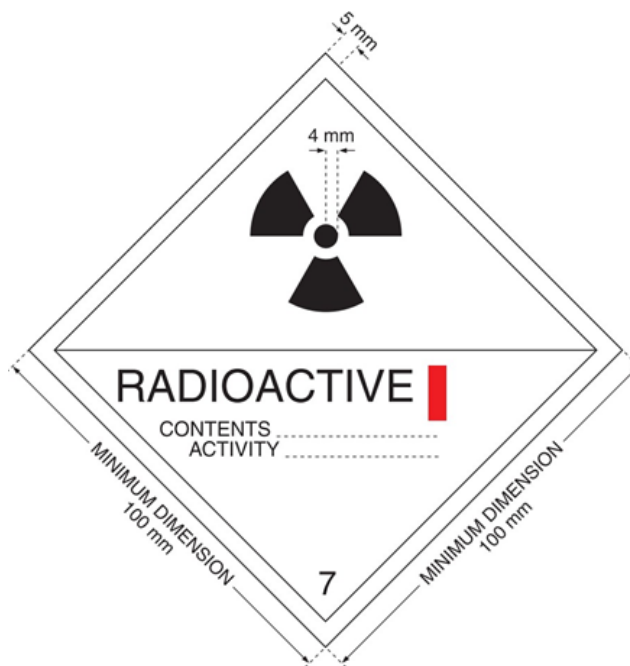
FIG. 2. Category I-WHITE label. There shall be a line inside the edge forming the diamond which shall be parallel and approximately 5 mm from the outside of that line to the edge of the label. The background colour of the label shall be white, the colour of the trefoil and the printing shall be black, and the colour of the category bar shall be red.
